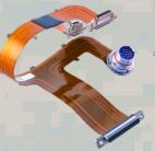
Integrated Flex / Rigid Flex **Circuit Assemblies**
