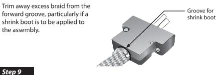
Visually inspect shield termination for problems. Correctly installed clamp must have full locking lip on all bands. If lip is damaged or missing, re-calibrate tool tension, check condition of cutter blade and knife, replace if worn or damaged.
