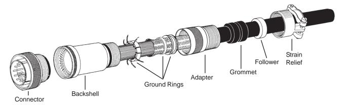
The following suggested procedure serves as a guide for the proper assembly and installation of Glenair EMI/RFI Environmental Backshells (Type E shield termination). It is recommended that trial samples of appropriate cables or harnesses be used to determine proper trim dimensions of the outer shield and individual conductors. This procedure is for the three ring style.
