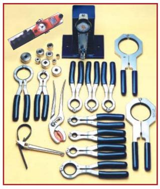
Glenair offers torque wrenches in two configurations. The hand-held torque wrench pictured above (top left), and the bench-mounted version (top center). Both are adjustable to a desired torque level of 20 to 360 inch pounds, and feature a 3/8" drive. A full range of receptacle and plug holders for Mil-Spec connectors and backshells is also offered.
