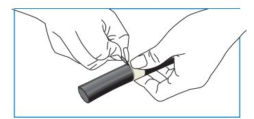
B) Score insulation lengthwise along the entire section of insulation to be removed.
