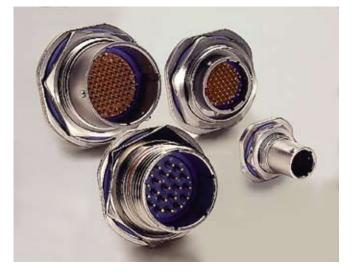
In hermetic connector manufacturing, the glass material is introduced either as separate glass beads or as a pre-formed glass seal insulator tooled to precise dimensions. The glass must be exactingly selected for each application according to its ability to form a strong bond with the metal materials.
