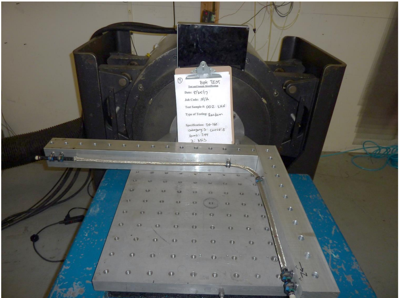
Figure 10: Vibration Test Set up for Z-axis
