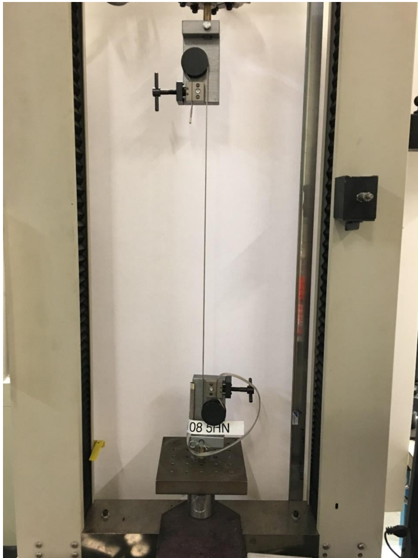
Figure 14: Pull Strength Sample Under Test
