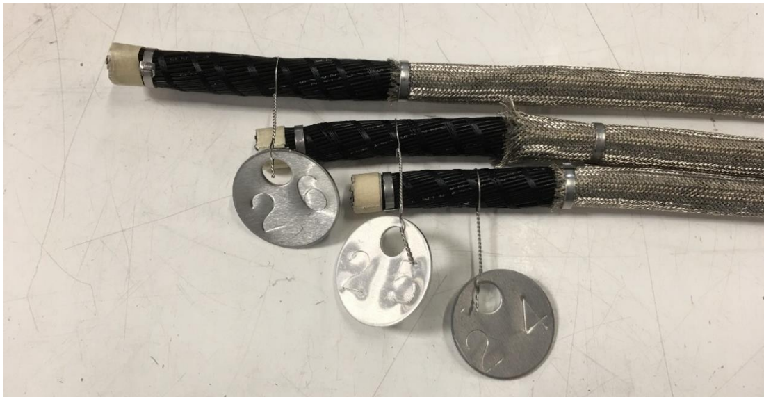
Figure 3: Armorlite braid samples installed on cable bundles and ready for testing
