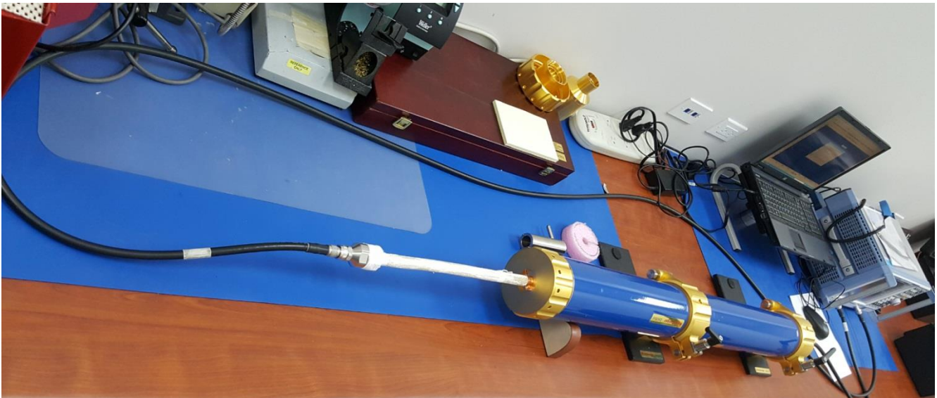
Figure 24: Screening Attenuation Test Setup Using bedea CoMeT 90 for 1 Meter Braid Assembly
