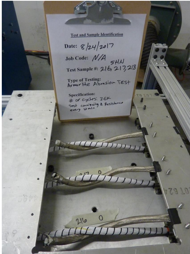
Figure 19: Abrasion Test Set up
