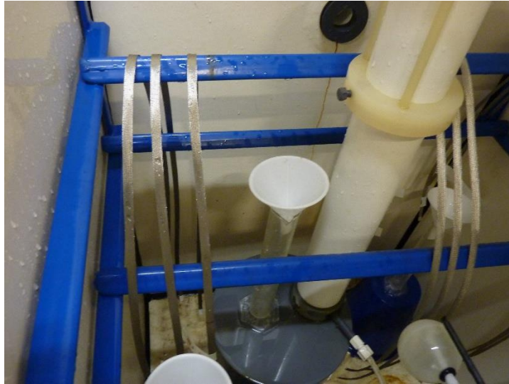
Figure 15: Placement of Samples in Salt Fog Chamber
