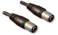
Overmolded threaded plug cordsets feature abrasion resistant extruded polyurethane jackets or ultraflexible nylon overbraid. Polyamide overmold, tinned copper braid shield. High strength silver-coated copper alloy conductors, crosslinked ETFE insulation. Wire size depends on contact size. Size #23 contacts have #24 AWG wire, 3 amp micropins have #26 AWG wire, and 1 amp nanopins have #30 AWG wire.
