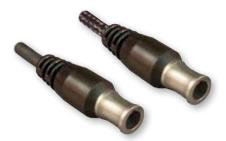
Overmolded Quick Disconnect receptacle cordsets feature abrasion resistant extruded polyurethane jackets or ultraflexible nylon overbraid. Polyamide overmold, tinned copper braid shield. High strength silver-coated copper alloy conductors, crosslinked ETFE insulation. Wire size depends on contact size. Size #23 contacts have #24 AWG wire, 3 amp micropins have #26 AWG wire, and 1 amp nanopins have #30 AWG wire.
