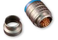
Series 881 threaded coupling, cable plug with solder cup contacts feature threadon rear adapters allowing access to solder cup contacts. Install cable shield braid directly to connector with Band-Master Micro band. Three contact sizes are available with current ratings of 5A, 3A and 1A. Aluminum or stainless steel housings, thermoplastic insulators. Ultraminiature SuperFly® connectors are ideal for soldier systems and other applications where ruggedness and field repairability is required.
