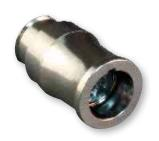
Series 880 Quick-Disconnect (QDC) in-line receptacles with solder cup contacts have thread-on rear adapter to allow access to contacts. Install cable shield braid directly to connector with Band-Master® band. Three contact sizes are available with current ratings of 5A, 3A and 1A. Aluminum or stainless steel housings and thermoplastic insulators. Ultraminiature SuperFly® connectors are ideal where ruggedness and field repairability is required.
