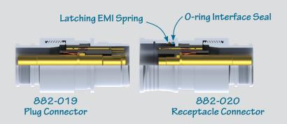
Push-pull SuperFly Datalink receptacle connectors feature a canted coil spring for secure mating and excellent EMI protection while fluorosilicone O-ring provides watertight sealing when mated.
