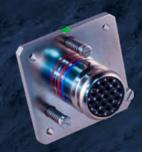
Assisted separation: Springloaded kick-off posts are designed to overcome contact separation force (normal force) with adjustable flange-mounted springs. Separation force may be calibrated IAW application requirements and insert arrangement.
