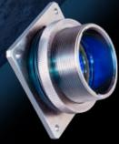
Assisted separation: Adjustment ring on receptacle shells provides reliable and repeatable calibration of assisted separation force. The adjustment ring interfaces directly with the spring-loaded kick-off posts on the plug. A set screw fitting locks the ring in place after adjustments have been made.
