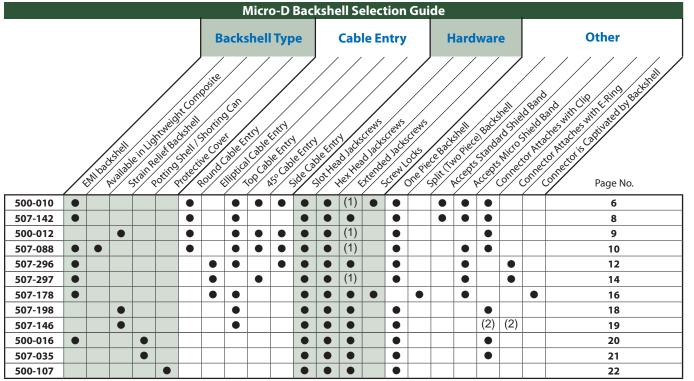
(1) Extended jackscrew will not work with 45° cable entry or with dual 45° entry backshells.
