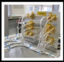
Turnkey satellite test harnesses and Electronic Ground Support Equipment racks
