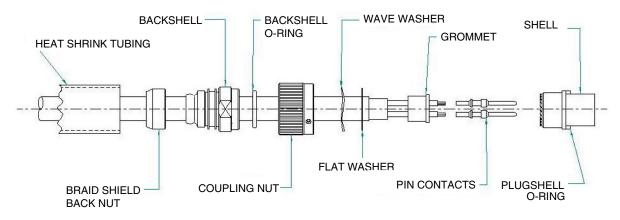
1) Strip off the cable jacketing pursuant to the dimensions shown on Table 8, being careful to not cut any of the wire strands comprising the braided shielding.
