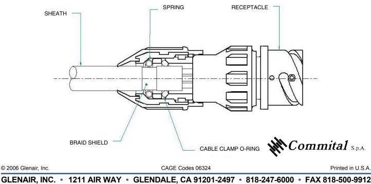
Figure 22: RG Type Wired Connector
