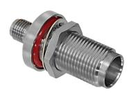
TNC Female / SMA Female. Jam nut panel mounting. Connect TNC plug to SMA plug with 852-163 adapter. Stainless steel body and hex nut. Gold-plated BeCu contact. Nickel-plated brass lock washer, PTFE insulator, silicone O-ring.
