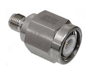
TNC Male / SMA Female. Connect TNC jack to SMA plug with 852-160 adapter. Stainless steel body with gold-plated BeCu contact, PTFE insulator, nickel-plated phos bronze lock ring, and silicone gasket.
