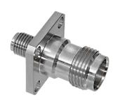
TNC Female / SMA Female. 4 Hole Flange. Connect TNC plug to SMA plug with 852-162 adapter. Stainless steel body, gold-plated BeCu contact, PTFE insulator.
