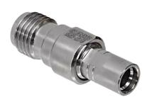
SMP Male / SMA Female. 852-174 adapter has smooth bore SMP male connector interface. Stainless steel body, gold-plated BeCu contact, PTFE insulator.
