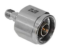
NMale/SMA Female. Connect N jack to SMA plug with 852-164 adapter. Stainless steel body with gold-plated BeCu contact, PTFE insulator, nickel-plated phos bronze lock ring, and silicone gasket.
