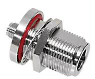
N Female / SMA Female. Connect N plug to SMA plug with 852-166 panel mount adapter. Nickel-plated brass body and hex nut. Goldplated BeCu contact. Stainless steel lock washer, PTFE insulator, silicone O-ring.
