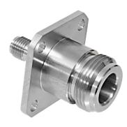
N Female / SMA Female. Connect N plug to SMA plug with 852-167 panel mount adapter. Stainless steel body, gold-plated BeCu contact, PTFE insulator.
