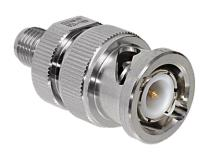
BNC Male / SMA Female. 852-189 adapter connects female BNC to SMA male connector. Stainless steel SMA body, nickel-plated brass BNC body and coupling nut. Gold-plated BeCu contact, PTFE insulator, nickel-plated brass wave washer. Silicone gasket.
