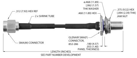
TOLERANCE IS: +1.80/-0.00 FOR "L" LESS THAN OR EQUAL TO 60.00 INCHES +3%/-0.00 FOR "L" GREATER THAN 60.00 INCHES
