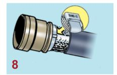
IMPORTANT: Always roll band through the buckle slot twice (see Step 3). Bands must be double-coiled to function correctly. The failure to roll the band through the buckle slot twice is the most common user error in band style terminations.
