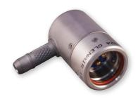
157-008 MIL-DTL-55116 type audio plugs feature 90° cable entry with an integrated, configurable 8-position backshell. 6 conductors accommodation with max  $\emptyset$  .045" insulation each. Available in both 5 pin and 6 pin configurations. Shells are made of passivated stainless steel, contacts are gold plated copper alloy. Plug connector contacts are sealed in the unmated condition.
