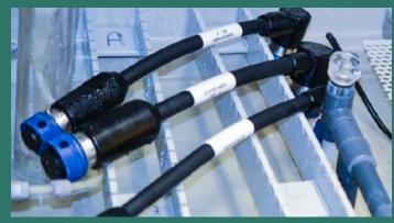
SuperG55 series cables undergoing qualification testing
