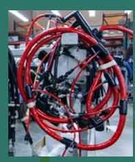
Glenair's hydrostatic test lab accommodates pressure testing of discrete connectors as well as large multibranch assemblies
