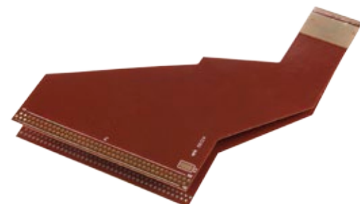
Selective bonding of discrete layers of flex circuitry
