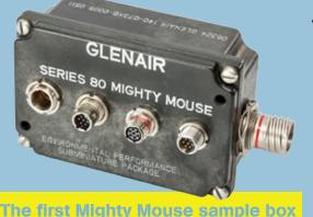
In 2005 we made our first demonstration box. Series 800, 801, 803, and 804 receptacles were mounted into the lid of a composite box. We added a 38999 connector in order to show the dramatic size reduction possible with the Mighty Mouse. Overmolded plugs were supplied with the box, allowing customers to mate and de-mate the four types of connectors.
