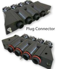
The Glenair IRT series is a rectangular power connector for harsh environmental conditions. Available with three, four and six contacts, typical for traction motor applications. Suitable for single cables AWG 4 – 373MCM (35 to 185 mmg). Working voltage up to 3000 Vcc. Two mating systems offered:
