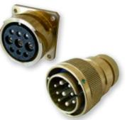
ITS-MB connectors are compliant with VG95234, using all the same insert arrangements available in the standard ITS Reverse Bayonet Connectors catalogue. Typically they are used for power and signal transmission, with wires from 26 AWG to 4/0. A wide variety of backshells allow the ITS-MB to accept jacketed cables, single or multi-poles, with or without RFI/EMI shielding, conduits with PG or metric thread. IP67 protection is the standard performance. IP68 on request.
