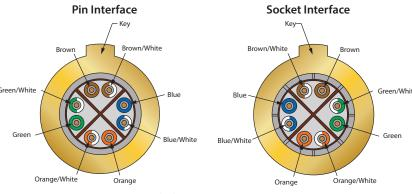
**Contact Performance Specifications Temperature Range** -55°C to +175°C **Environmental** IAW connector specification Sealing **Corrosion Resistance** 48 hours salt spray Fire, Smoke and IAW FAR 25 **Toxicity EMI Shielding** 360° shielding for each pair **Nominal Current** 1Amp **Contact Resistance** Max 60 milliohms Wire IAW TIA/EIA Cat 6A and ISO EA **Mating Cycles** > 500 DWV 500 VAC RMS sea level
