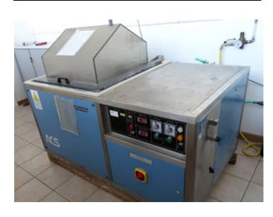
**Accelerated harsh-weather testing** is performed to ensure components under test meet qualification requirements for galvanic corrosion and resistance, resistance to solvents, and SO2.
