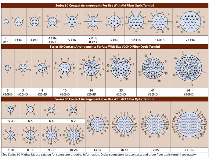
Cavity numbers are mating face view of pin connectors.
