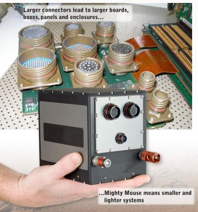
lower density contact arrangements lead to fatter and heavier interconnecting cables, including increases in accessory hardware size, and the amount of shielding and jacketing material required.
