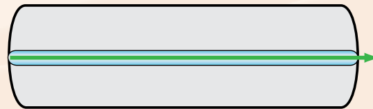
A singlemode fiber has a much thinner core than a multimode fiber. Light pulses follow a single direct path. Bandwidth essentially approaches infinity—limited practically to about 100,000 gigahertz.
