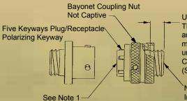
Uncontrolled Thread Size and Length may extend under the Coupling Nut (See Note 2)
