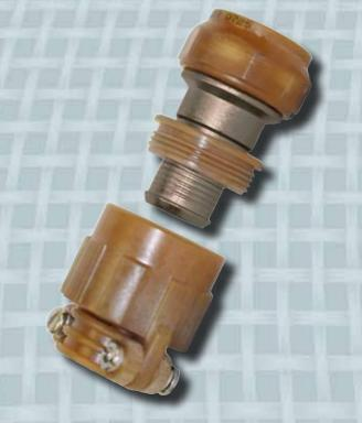
Thermoplastic connector components, such as this Band-in-a-Can Backshell, may be selectively plated with conductive material. This strategy enables users to enjoy the weight saving and durability properties of composites while addressing EMC grounding requirements.
