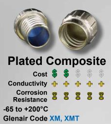
Plated composite connectors and accessories provide unsurpassed compliant corrosion protection and excellent conductivity. Glass-reinforced thermoplastic is metallized and plated with electroless nickel (Glenair Nickel-PTFE is also now available). Plated composite connectors and accessories have become the first choice for aerospace programs seeking to eliminate cadmium and reduce weight.
