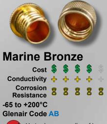
Marine bronze, an alloy of bronze, aluminum and nickel, is more compliant resistant to the corrosive effects of seawater than ferrous alloys. Used on Glenair's GeoMarine connector coupling nuts, marine bronze is unplated and develops an aluminum oxide protective layer when exposed to air. Marine bronze connectors and accessories are found in shipboard and offshore drilling applications.
