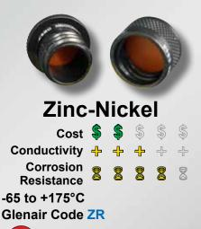
Recently added to MIL-DTL-38999 and MIL-DTL-83513, this "Class Z" *Compliant* zinc-nickel plated aluminum has become a cost-effective alternative to cadmium. Available with a black RoHScompliant chromate conversion coating, zinc-nickel plated aluminum is commonly found on soldier systems and military airframe applications.
