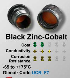
Zinc-cobalt with black trivalent chromate topcoat fills the need *Compliant* for a RoHS compliant conductive black finish for soldier systems, unmanned vehicles, robots and other tactical gear. This new addition to the Glenair lineup is likely to replace black zinc-nickel for new Future Combat System applications. Black zinccobalt plating is a standard finish on Glenair's ITS 5015 reverse bayonet power connectors.
