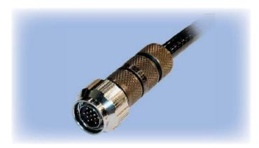
New Series 80 Backshells, available for all "Mighty Mouse" style connectors, feature multiple o-ring seals for environmental protection as well as an EMI shield ring for reliable grounding of cable shields and screens.
