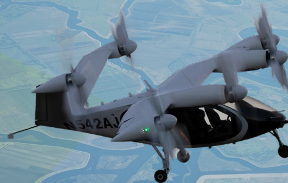
Anhedral Tip rotor design (above). The Joby S4 (left) utilizes an Anhedral Tip for performance and noise reduction.
