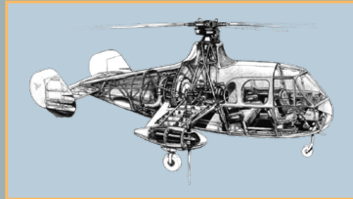
Schematic drawing of a prototype Fairey Gyrodyne rotorcraft from 1946
