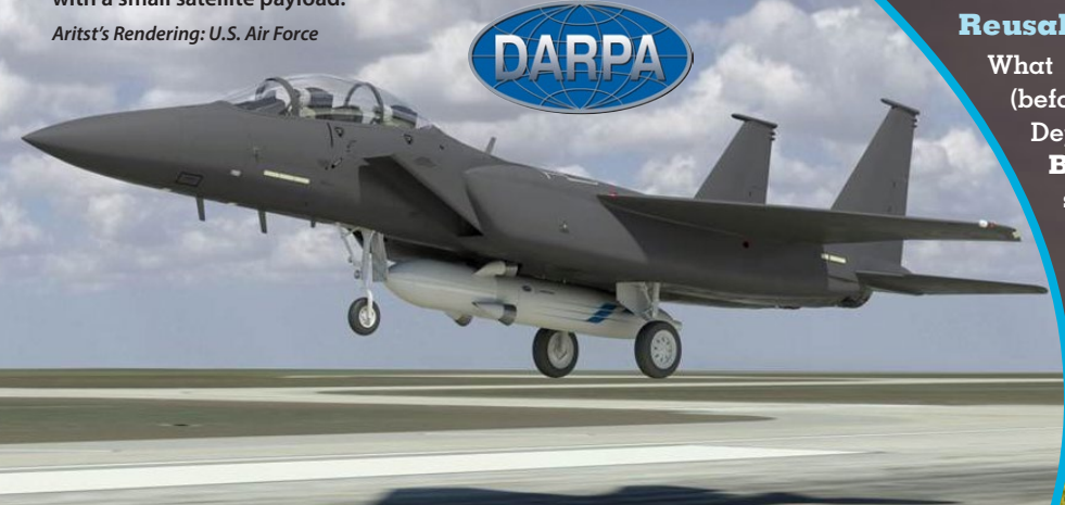
The ALASA Airborne Launch Assist Space Access uses an F-15 fighter jet as the "first stage" to launch an expendable vehicle with a small satellite payload.
