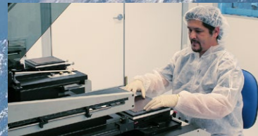
Space-Grade Clean Room for Interconnect Assembly
