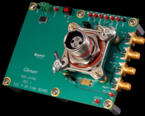
MIL-DTL-38999 type 2.5mm Elio® compatible transceiver evaluation board
