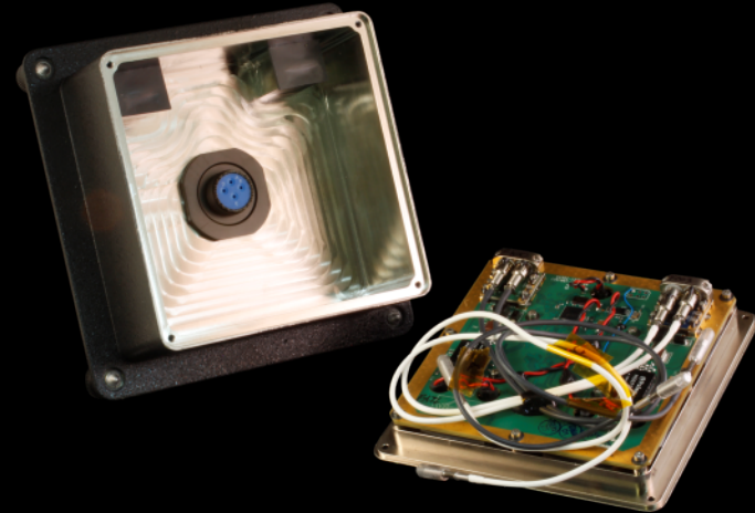
Small form-factor opto-electronic media converter with field fault monitoring
