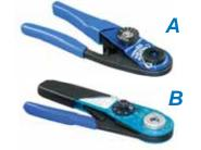
A Standard M22520/2-01 crimper. Use with standard size #23 "Mighty Mouse" contacts and with M39029/76 and /78 coaxial center contacts. Requires positioner, ordered separately. **B** Special MH992 crimper used with 50 ohm matched impedance coaxial inner contacts. Requires positioner, ordered separately.
