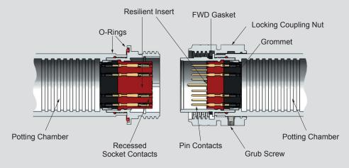
Receptacle (left) and Plug (right) connector pair
