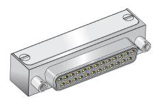
Low profile right angle PC tail HiPer-D® socket connectors feature rugged machined aluminum shell and aluminum alloy cover for improved EMI protection. Contacts are non-removable size, #20 or #22. Intermateable with standard M24308-type D-Subminiature connectors, the HiPer-D® features epoxy potting for environmental sealing. Threaded holes on the rear of the connector allow attachment to circuit board. Glass-reinforced thermoset epoxy insulators. 1000 VAC, 5 Amps (#22) or 7.5 Amps (#20).
