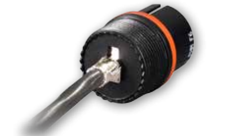
Push terminated USB connector into the dielectric until the tab bottoms in the notch
