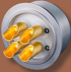
Considered the "Granddaddy" of all connector specifications, MIL-DTL-5015 covers power connectors available in contact sizes ranging from #16 up to #0. Operating voltages range from 200 up to 3000 volts AC (rms).
