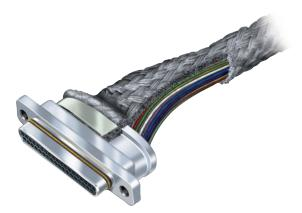
Cross-sectional view of a Micro-D connector assembly optimized for EMI noise suppression. Note the use of braided shielding, shield termination band and EMI ground spring. Effective EMI noise suppression may be accomplished solely with the use of filter connectors, but many designers prefer to augment the noise suppression provided by filters with accessory hardware such as banding backshells, conductive gaskets, gounding studs and cable shielding.
