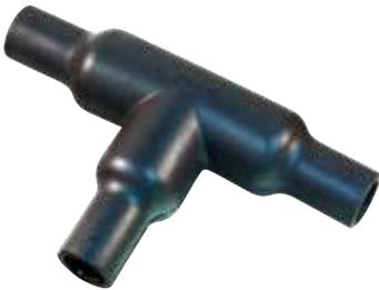
Low profile “Tee” heat shrink transitions provide an easy to install and rugged cable routing solution. Transitional boots are available in eight material options with five adhesive choices. All Adhesive lined and unlined shrink books are RoHS compliant. Transitional boots are water-tight when equipped with factory installed or user-installed adhesive. Choose boot size based on cable diameter.
