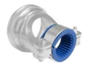
Rubber bushing strip fits under strain relief saddle bars and provides cushioning and protection to wire bundle. Use with full radius saddle clamp strain reliefs including 620-038, M85049/118, /120, /121, /123, /124, and /126. These 10 inch (254 mm) strips are available in three widths to fit small, medium and large width saddle bars. Trim to desired length with scissors. Blue silicone rubber.
