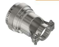
saddle clamp fits Series 80 Mighty Mouse connectors. Clamp has enlarged inside diameter and longer frame to provide clearance for size 8 coax/twinax/quadrax/octaxial contacts with sealing boots. Extra clearance helps prevent contact splay and damage. Full radius saddle bars have self-locking SST clinch nuts. Anti-decoupling mechanism provides audible detented coupling and prevents backoff under high vibration.
