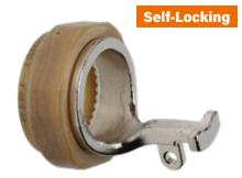
*Lightweight, self-locking, conductive.* 450H\*030 Qwik-Ty clamps fit MIL-DTL-38999 Series III and IV connectors. Metallized composite Qwik-Ty has ground lug for attaching a ring terminal with #4 screw. Anti-decoupling mechanism provides audible detented coupling and prevents backoff under high vibration. Secure wire bundle with plastic strap or lacing tape (not included).
