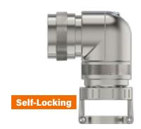
Individual shield termination. Self-locking. 400HD011 backshell fits MIL-DTL-38999 Series III and Series IV connectors. Spin coupling, non-environmental. Grounding ring has slots for individual cable shields. Anti-decoupling mechanism provides audible detented coupling and prevents backoff under high vibration. Coupling nut, adapter and ground ring are aluminum alloy. Gold plated copper alloy ground spring, PTFE washer. Saddle clamp is aluminum alloy with stainless steel hardware.
