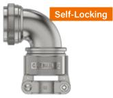
*EMI shielding. Self-locking. Straight, 45° or 90°.* 380V\*143 backshells fit Glenair Series 806 connectors. Two ground rings for terminating individual and overall braid shields. Anti-decoupling mechanism provides audible detented coupling and prevents backoff under high vibration. Non-environmental. Type H heavy duty saddle clamp has stainless steel telescoping fillister head screws and lockwashers. Available in aluminum or stainless steel.
