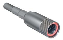
Black zinc plated aluminum alloy backshell fits CB Series connectors with M14 x 1 threads. Black nitrile bushing provides flexible cable strain relief and cable sealing. Cut tapered bushing to fit varying cable diameters. Supplied unassembled with two O-rings and aluminum alloy ground ring. Maximum weight 15 grams.
